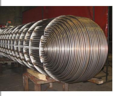
**Delta Tee** is a leading manufacturer of Shell & Tube heat exchangers in the USA. These units are very rugged and see service in the Petro-Chem, Power and Oil & Gas sectors due to their ability to accommodate high pressures and temperatures. Industrial Refrigeration is also well served by Shell & Tube chillers and condensers, working as low as -55°f.
