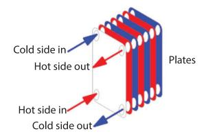
Plate & Frame exchangers are efficient, smaller than Shell & Tube, and are easily cleaned. Access room around the units is reduced and the capacity can be expanded within their original footprint.
